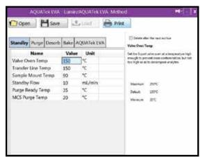
**Method Development Screen** - Load default water, soil, and methanol extraction methods for common applications or optimize parameters for specific sample types. Standby, Purge, Desorb, and Bake Tabs allow efficient review and revision of parameters. Parameter description and useful information are shown to the right of the tab.
