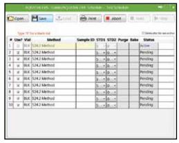
Schedule Screen - Schedule building is easier than ever thanks to excel-based features such as highlight, fill down and fill sequential commands. Schedules can be edited at any time, even while running. This allows for priority samples to be added in at any time. Schedule screen also includes useful fields such as sample ID, Internal standards addition, and vial position. Lastly, the schedule captures essential information such as purge and bake pressures, and sample status.
